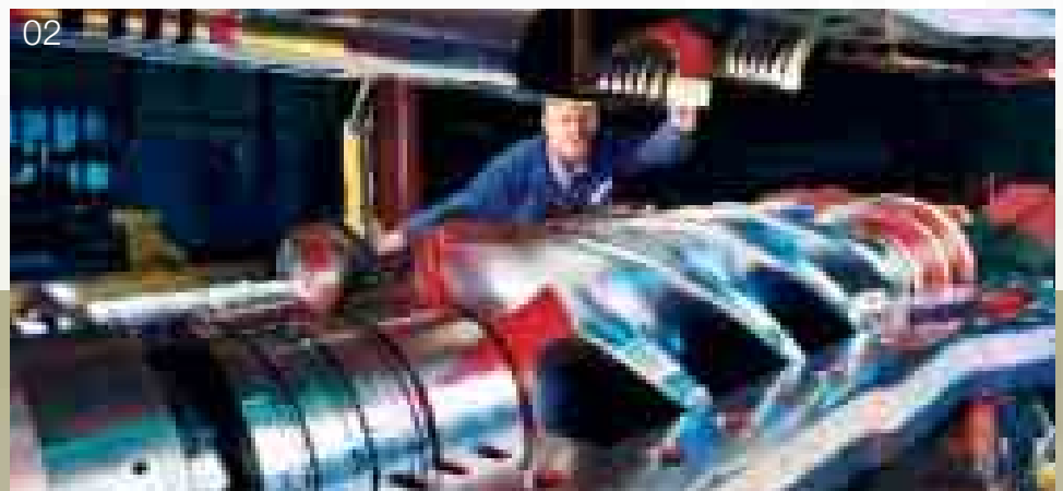
02 Assembly of SKUEL643 process-gas screw compressor
