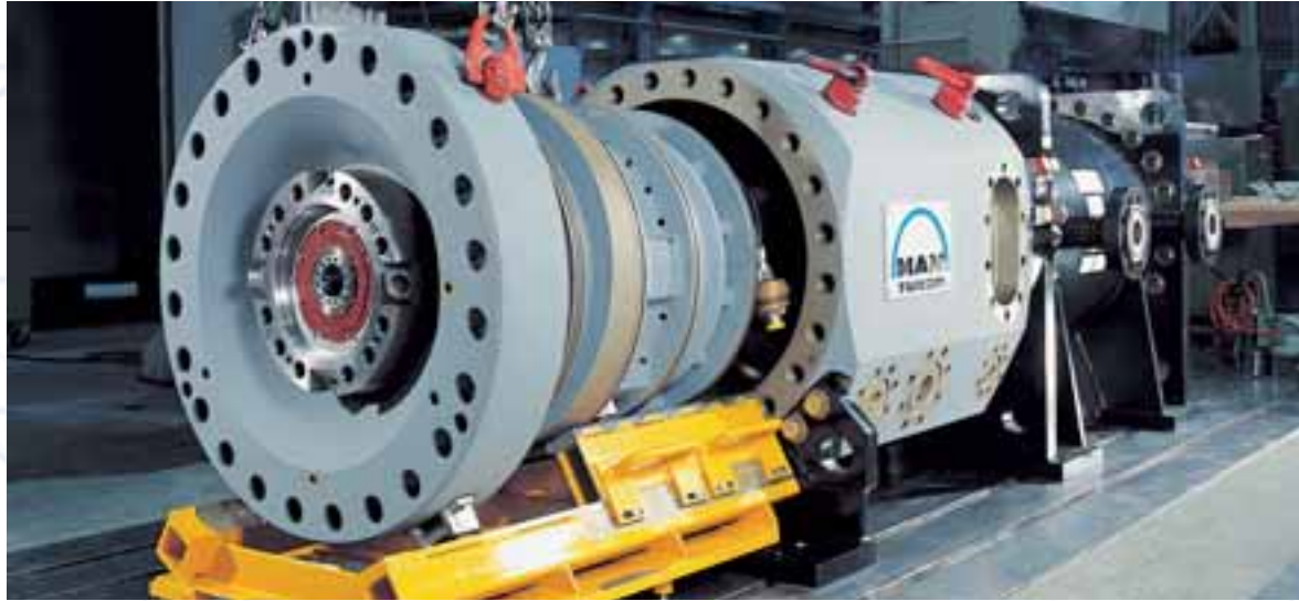
HOFIM Sealed – hermetically closed, oil-free compressor for high-pressure applications
